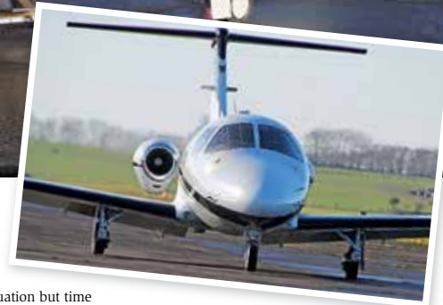
Above: with no reverse thrust and (at least for the time being) no anti-skid brakes, care must be taken on landing
